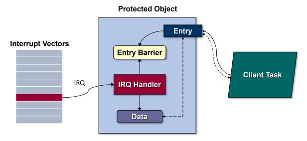
The interrupt handler stores data within the PO and only enables the entry barrier when ready to either produce it or consume it via the entry parameters. The dashed lines in the figure represent this data flow.
