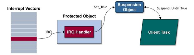
The language requires the run-time library implementation to allow calls to Set\_False and Set\_True during any protected action, even one that has its ceiling priority in the Interrupt Priority range, so this approach will work for interrupt handlers as well as tasks.
